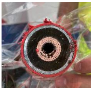
Figure 3 Cross section of cables cleaned in test
