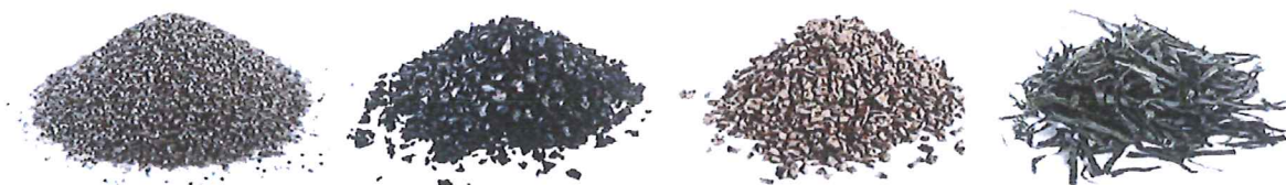
Figure 2: Products (sand, rubber granulate, backing, grass fibres (polyethylene)).
